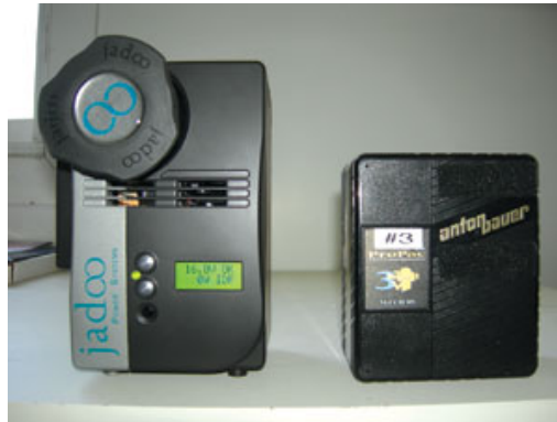
Both the N-Gen and a standard battery weigh about 5 pounds. The N-Gen is definitely bulkier, though.
