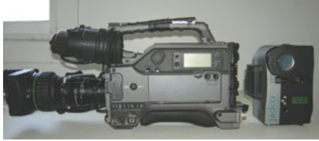
The Jadoo fuel-cell system uses industry-standard Anton/Bauer Gold Mount interfaces to attach to the rear of a video camera. But as I found out, one size does not fit all.
