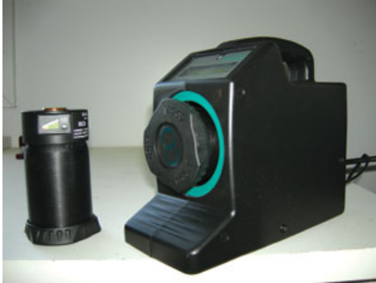
Ready for refill. The N-Stor cartridge clicks right into the FillOne station. In my tests, it took about 2 hours to top off a cartridge.
