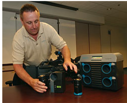
Larry Bawden, co-founder of Jadoo Power Systems, shows a hydrogen fuel cell device designed to replace standard batteries for video cameras used by television stations. Bawden sees a huge global market for the device. Sacramento Bee/Jay Mather
