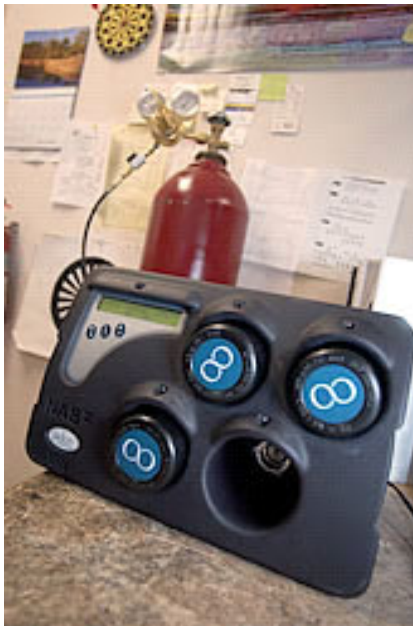
Above is a fuel-cell charging station, with a hydrogen tank in the background.
